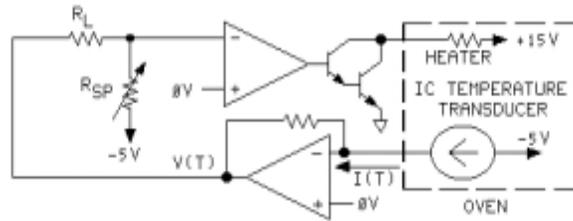
Figure 2. Simplified IC Transducer Circuit
