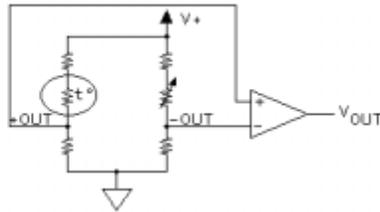
Figure 3. A Thermistor in a Wheatstone bridge arrangement
