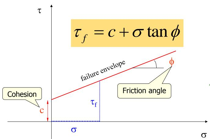
$\tau_f$  is the maximum shear stress the soil can take without failure, under normal stress of  $\sigma$ .
