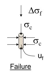
At failure,  $\sigma_3 = \sigma_c$ ;  $\sigma_1 = \sigma_c + \Delta \sigma_f$  $\sigma_3' = \sigma_3 - u_f$ ;  $\sigma_1' = \sigma_1 - u_f$
