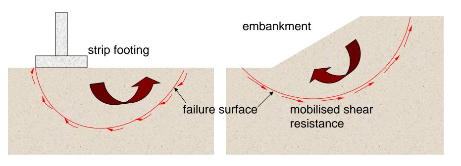
At failure, shear stress along the failure surface reaches the shear strength.
