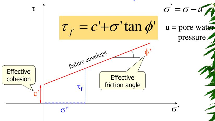
$\tau_f$  is the maximum shear stress the soil can take without failure under normal effective stress of  $\sigma$ .
