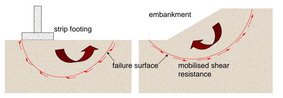
At failure, shear stress along the failure surface reaches the shear strength.
