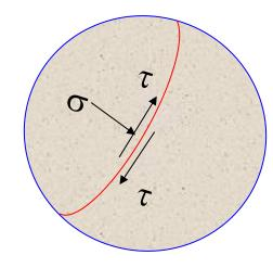
At failure, shear stress along the failure surface  $(\tau)$  reaches the shear strength  $(\tau_f)$ .
