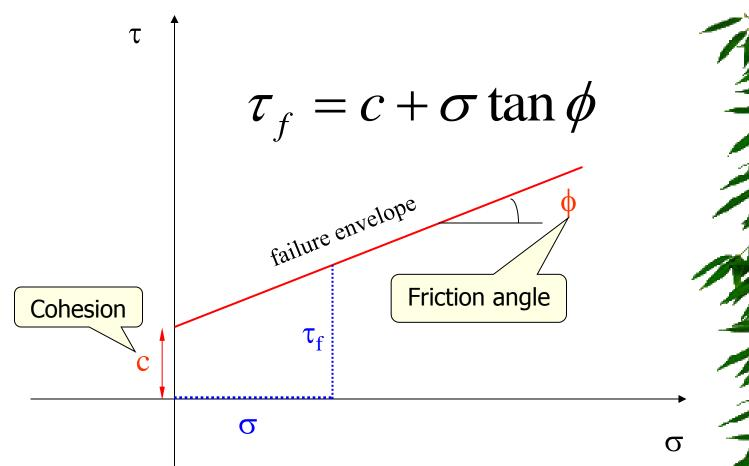
$\tau_f$  is the maximum shear stress the soil can take without failure, under normal stress of  $\sigma$ .
