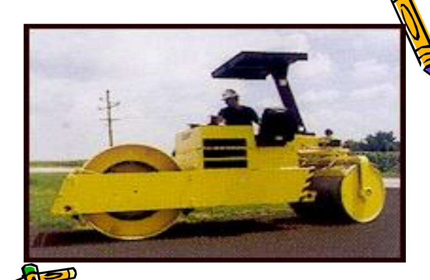
Fig. 1: Example of mechanical modification (Drum Rollers)
