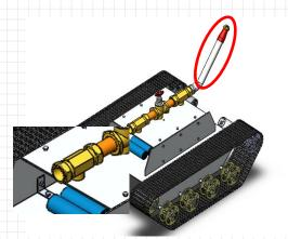
This hose is then connected to the body of the unmanned ground vehicle via valves. This valve then connects it to the water nozzle which in turn will shoot water out, extinguishing the fire.
