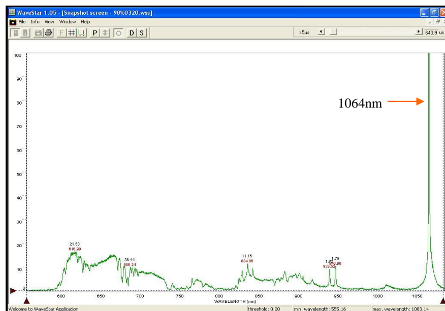
Figure 2: Spectrum of Nd:YAG laser with dominant line of 1064nm
