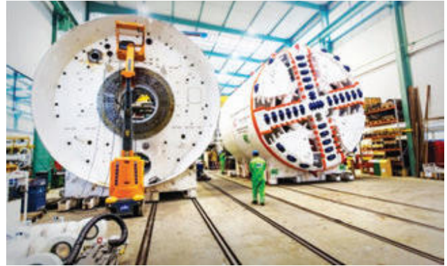
MRT Line 1 Tunnel Boring Machine under construction
