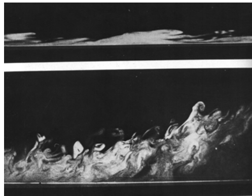
Adverse pressure gradient over the plate
