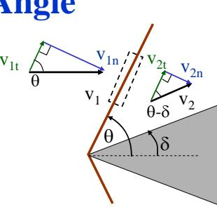
(from VII.23)  $\frac{v_{1n}}{v_{2n}} = \frac{(\gamma+1)M_1^2 \sin^2 \theta}{(\gamma-1)M_1^2 \sin^2 \theta + 2}$  (from geometry)  $\frac{v_{1t}}{v_{2t}} = \frac{v_{1t} \tan \theta}{v_{2t} \tan(\delta - \theta)}$
