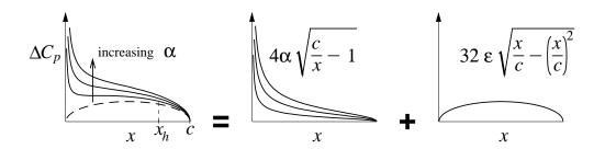
Define  $x_h$  as the location of the flap hinge, so the flap extends from  $x = x_h$ , to the trailing edge at x = c. The corresponding  $\theta$  locations are  $\theta = \arccos(1-2x_h/c) \equiv \theta_h$ , and  $\theta = \pi$ , respectively. The load/span and moment/span coefficients on the flap hinge can now be computed by integrating the pressure loading.
