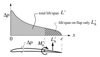
The loading  $\Delta p$  is directly related to the vortex sheet strength  $\gamma(x)$ , and can also be given in terms of the dimensionless pressure coefficient.
