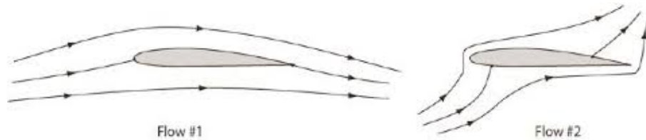
Figure 3: Kutta condition occurs in Flow # 1
