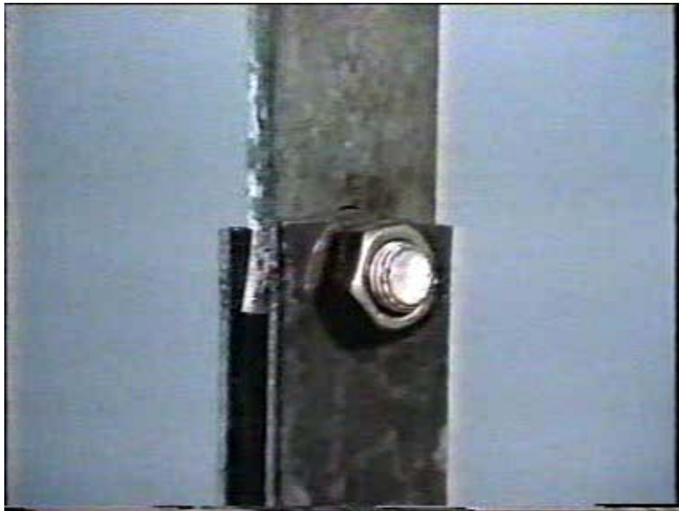
plate failure – end plate
