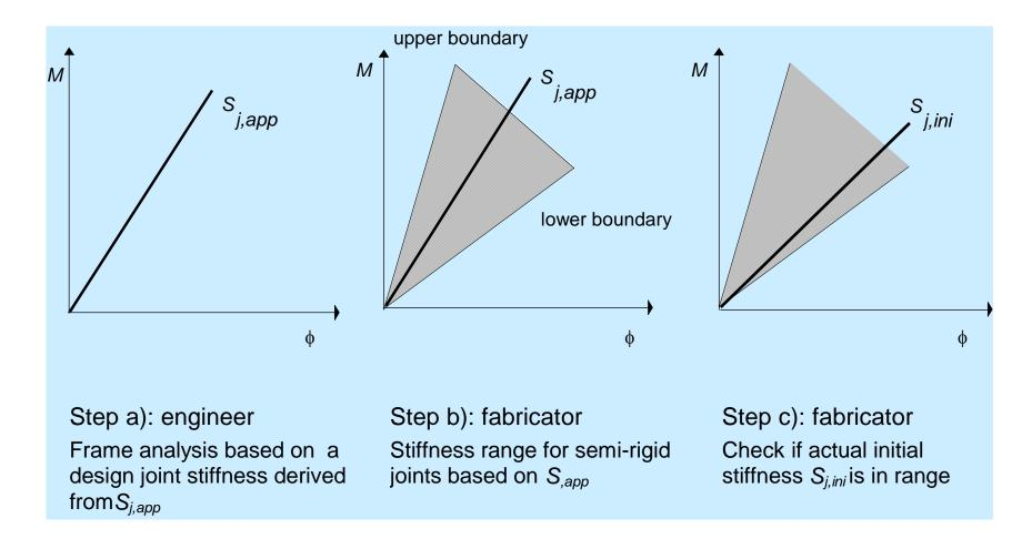
Semi-rigid joint stiffnesses can vary within a fairly wide range without significantly altering the frame resistance
