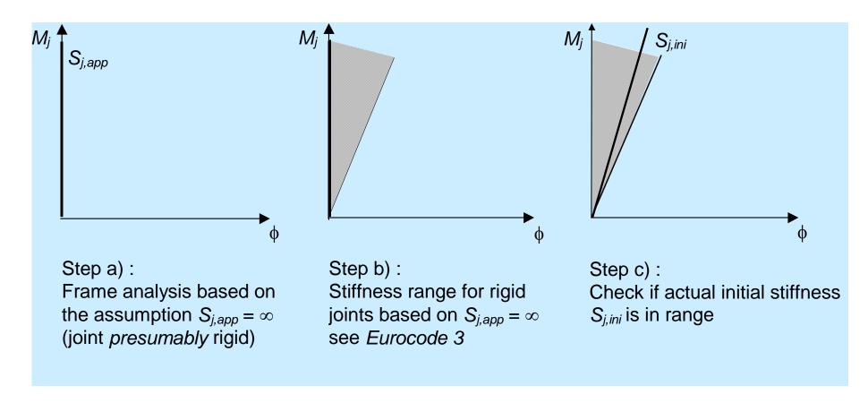
Joint must meet "rigid joint" classification criteria
