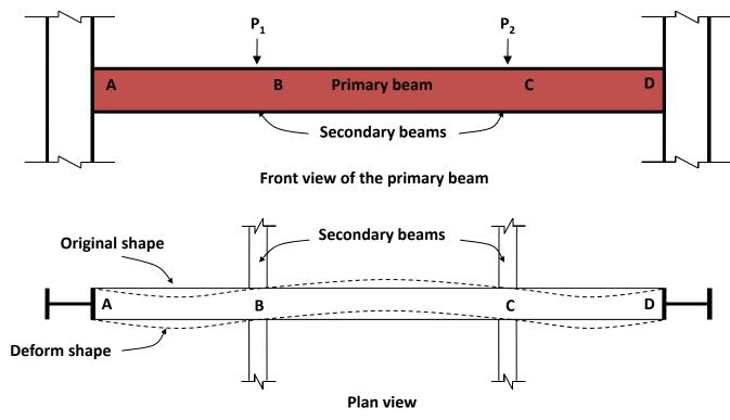
Points A, B, C and D are restrained from deform laterally by the secondary beams and the connection at column
