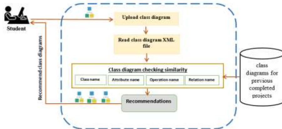
Figure 1: Overview of Class Diagrams Recommender
