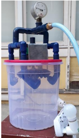
Rajah 2.2: Kit turbin hidro pico UTM
