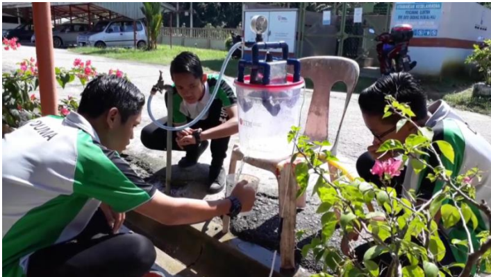
Rajah 5.5: Kaedah mengukur kadar alir air.
