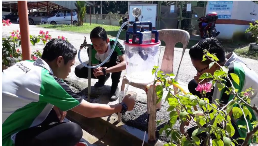
Rajah 14. Kaedah mengukur kadar alir air.
