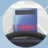
3 Still lacking a reaction, the system mildly applies the brakes. Should this too fail, the system activates the emergency braking and does everything possible to stop the truck.
