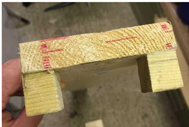
A flattening jig helps achieve a consistent taper on your pipes
