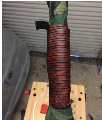
Bow with a leather handle, arrow rest and camo tape finish
