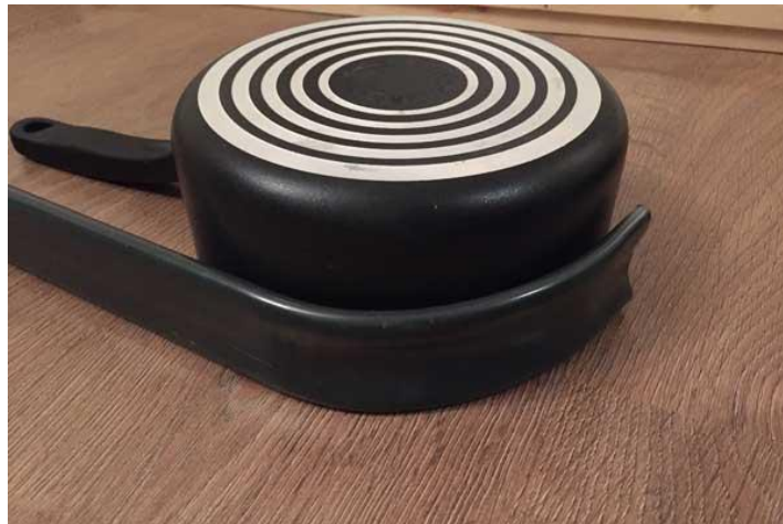
Forming the recurves – notice the dips created as the pipe is bent
