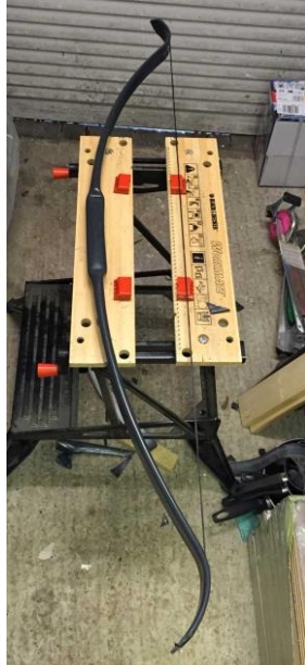
The finished bow with correct string – slightly stiffer lower limb evident
