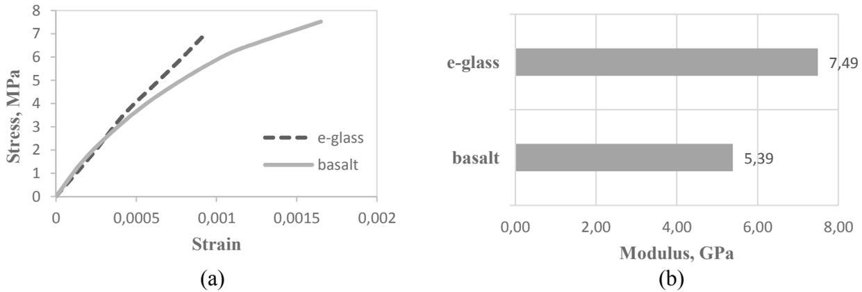
Fig. 2 Results comparison (a) Tensile Stress (b) Elastic modulus
