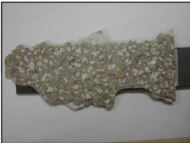
Fig. 21. Failure mode dominated by concrete shear failure.
