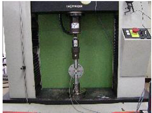
Fig. 10. Set-up of Arcan fixture to the loading machine.
