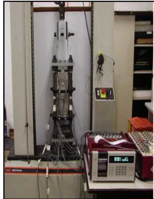
Fig. 6. Pull out test set up.
