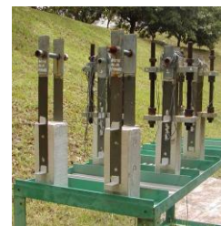
Fig. 9: BOLTALS50 specimens under six and twelve month exposure to outdoor environment
