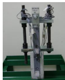
Fig. 8: Part of the BOLTALS50 specimen under six6 month exposure to laboratory environment
