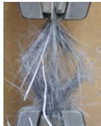
Figure 5: Mode of failure of the CFRP plate
