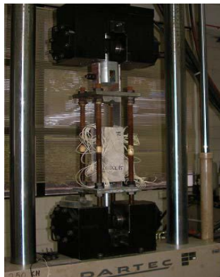
Figure 4: Testing of CFRP-Concrete prism
