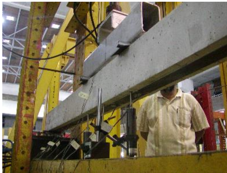
Fig. 2.22: CFRP Plate (black strip) externally bonded to tension face of reinforced concrete beam [40]
