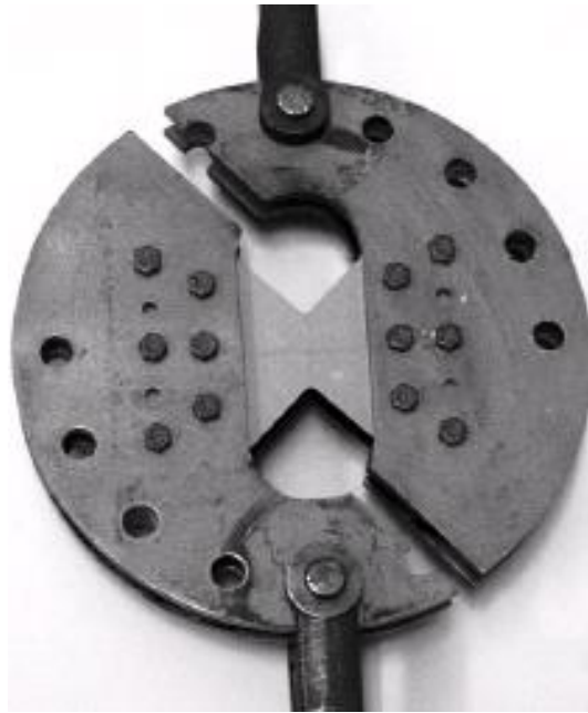
Fig. 2.43: Modified test fixture and butterfly specimen set-up by Yen et al. [63]
