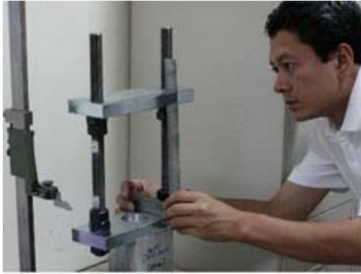
Fig. 3.17 (a): Setting-up stressed rig configurations
