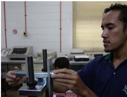
Fig 3.17 (c): Inserting high tensile steel bolt into CFRP Plates-end tabs holes
