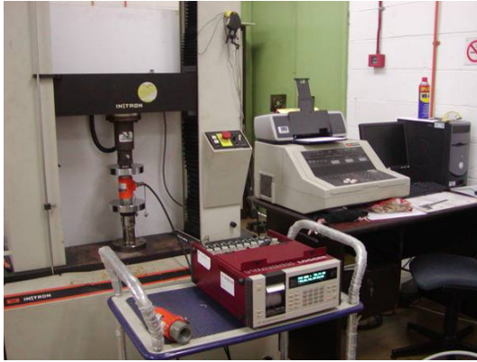
Fig. 3.15 (a): 50 kN load cell calibration under compression load using 100 kN Instron Universal Testing Machine
