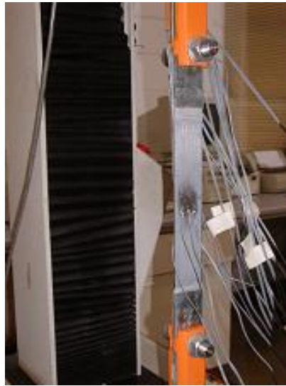
Fig. 3.10: Test set-up for determination CFRP plate-mild steel end tabs bond strength
