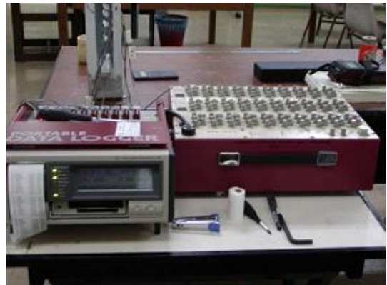
Fig. 3.17 (j): Strain output print-out in 30 minutes time interval for 24 hours monitoring duration
