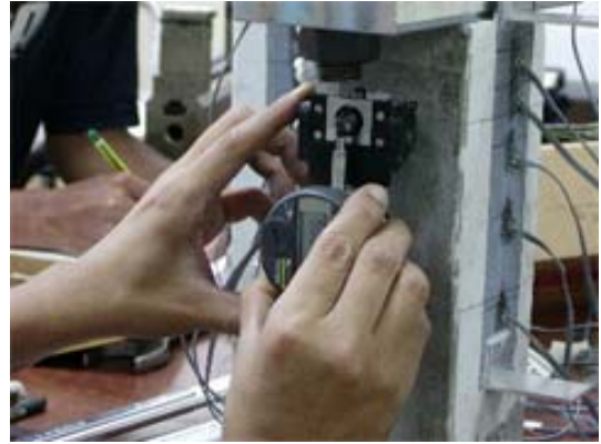
Fig. 3.17 (h): Measuring the strain of concrete during pre-stressed using digital Demec Gauge instrument
