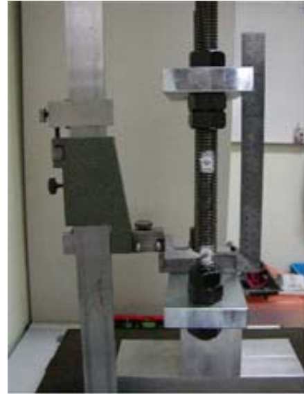
Fig. 3.17 (b): Upper and lower steel plates height calibration and measurement
