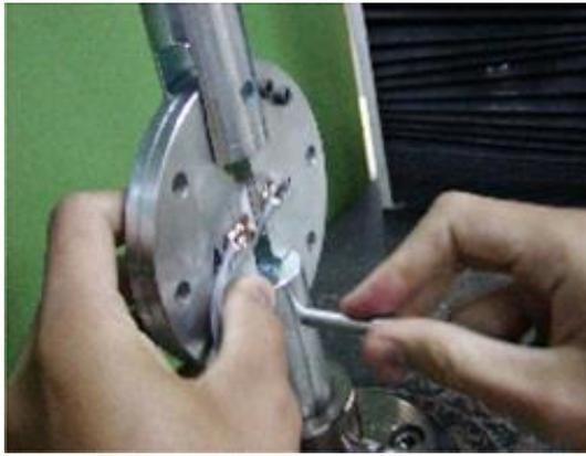
**Fig. 5.20 (a):** Attachment grip to holder by pin
