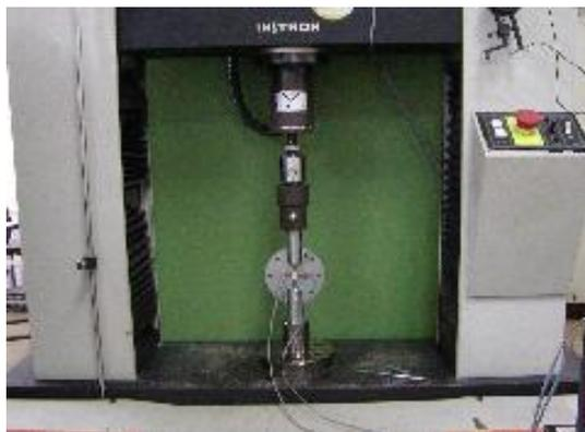
**Fig. 5.22 (a):** Completion set-up of Arcan fixture to the loading machine
