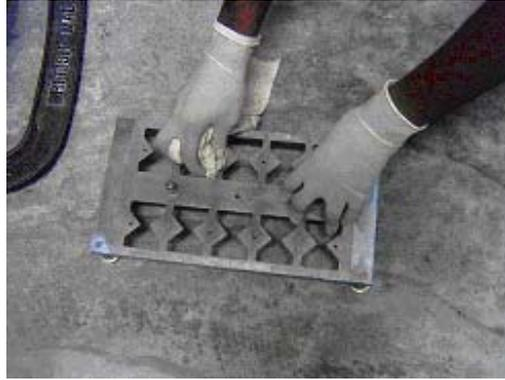
**Fig. 5.6:** Cleaning the mould using soft cloth with Carnauba wax
