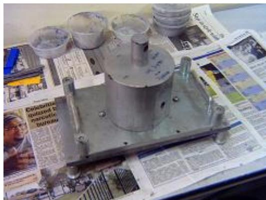
**Fig. 5.10:** A weight used to press the female part from top side
