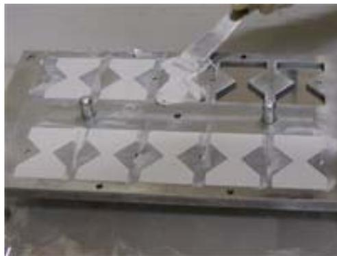
**Fig. 5.8:** Filling the epoxy mixture into the mould cavity
