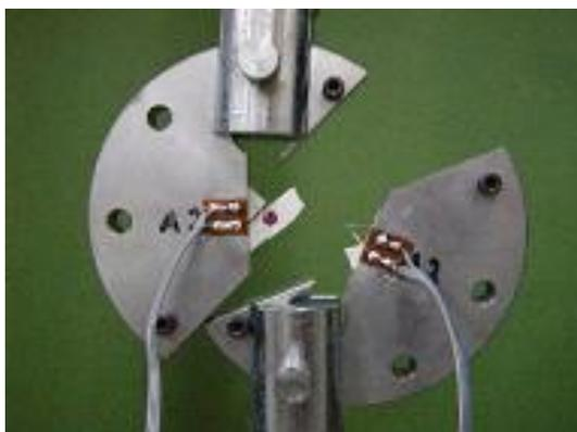
**Fig. 5.32 (a):** Specimen ESLT-OD01 just after failure
