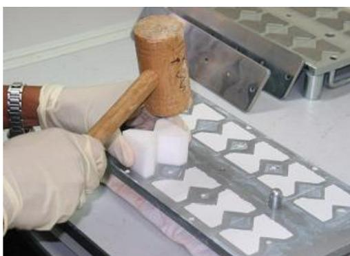
**Fig. 5.11:** Specimen demoulding using Teflon block and wood hammer
