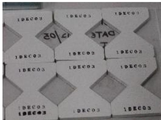
**Fig. 5.13:** Specimens ready to be exposed
