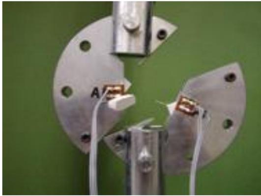
**Fig. 5.34 (a):** Specimen ESLT-PW01 just after failure
