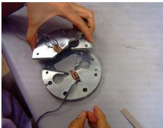
**Fig. 5.17 (a):** Arcan male grip attached onto female grip
