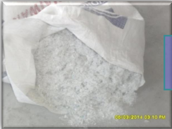
Recyclates or recycled glass fibre or Raw rGF
