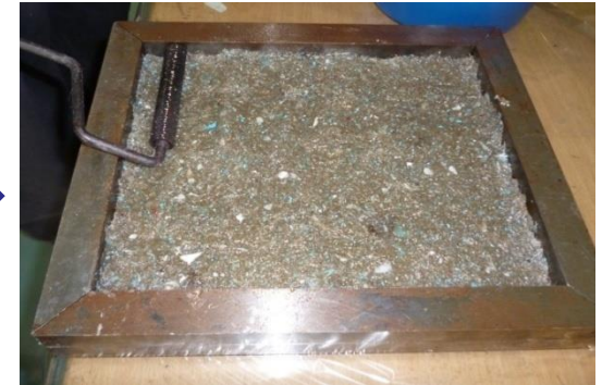
Resin poured into the mould and distributed by roller
