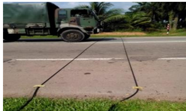
Figure 2 Pneumatic Tubes are 1 Metre Apart
