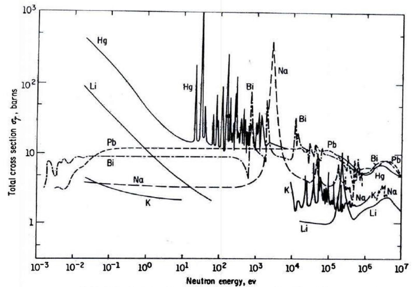
FIG. 10-1. Total neutron cross sections of some liquid metals.
