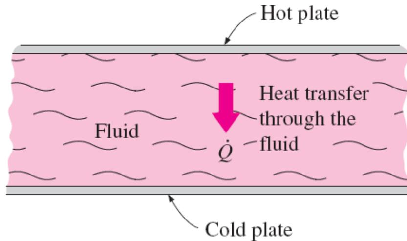
Heat transfer through a fluid sandwiched between two parallel plates.
