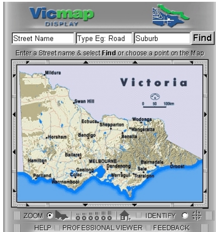
Figure 20: VicMap Display utilising server-side scripts to produce dynamic maps
