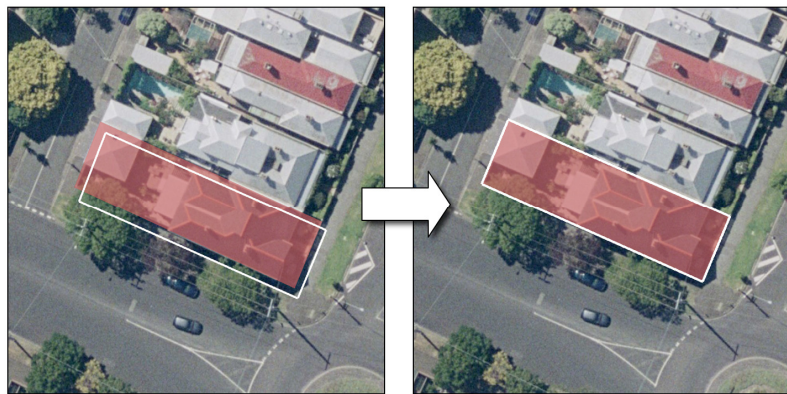
Figure 2. Cadastres will be survey accurate: virtual representations must match reality
