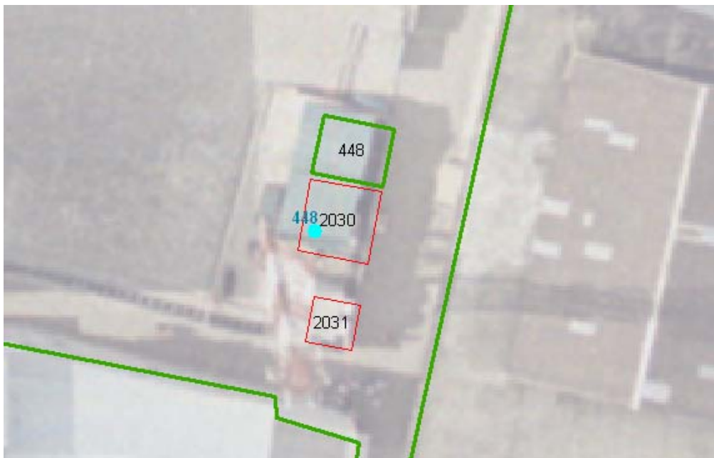
Figure 5-4 The centroid point coordinates in core database are wrong for building no. 448
