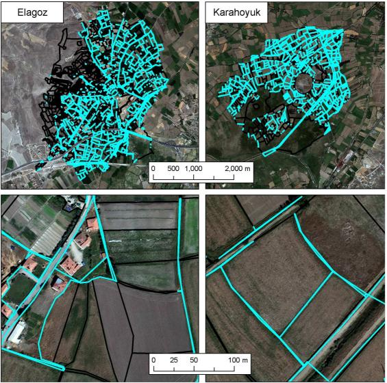
Figure 4. Linear and/or small area errors on overlapped data (with no/default XY tolerance): All errors within whole data in two districts (above), errors in specific areas (below).
