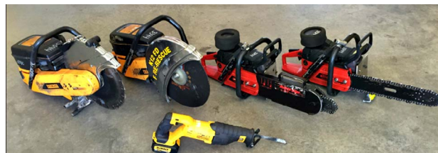
Fig. 2. Fire-fighters various types of saws, roof chainsaw, K-12/Partner (rotary) saw, standard chainsaw, and/or a reciprocating saw.
