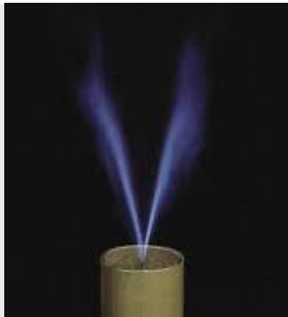
Schematic illustration of an instantaneous picture of a “V-shaped” turbulent premixed flame stabilized by a bluff-body
