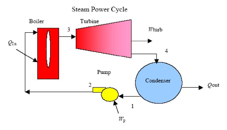
The working fluid, steam (water), undergoes a thermodynamic cycle from 1-2-3-4-1. The cycle is shown on the following *T-s* diagram.
