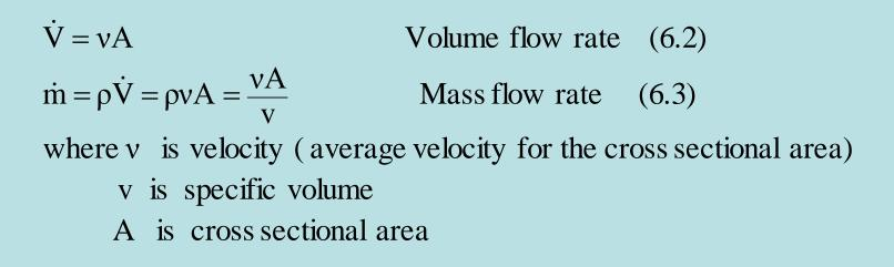
For steady flow and single inlet and single outlet, continuity equation becomes:
