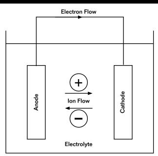
Electrical current flows through the electrolyte to balance the flow of electrons in the metal. In this case, the carriers of the electrical current are ions in the electrolyte. Anions (negatively charged ions) flow toward the anode and cations (positively charged ions) flow toward the cathode. Figure reproduced from NACE International Basic Corrosion Student Manual, p. 2.9.
