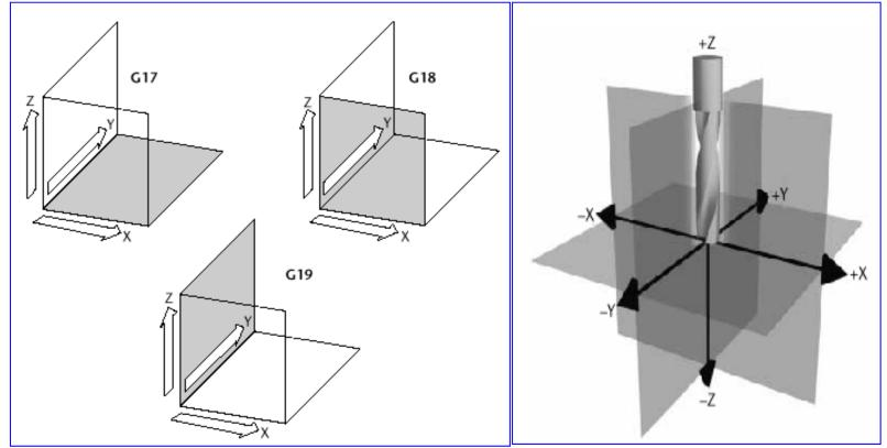
The three planes in the Cartesian coordinate system are **XY**, **XZ**, and **YZ**. These are referred to as **G17**, **G18**, and **G19**, respectively, on the mill.
