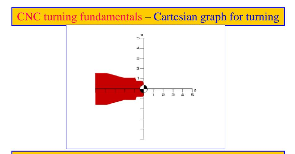
When measuring X and Z coordinates, use a central reference point. Start all measurements at this reference point, the origin point (X0, Z0). For all our examples **the origin is located at the center right-hand endpoint of the workpiece**. Keep in mind that at times the center left-hand endpoint of the workpiece may be used
