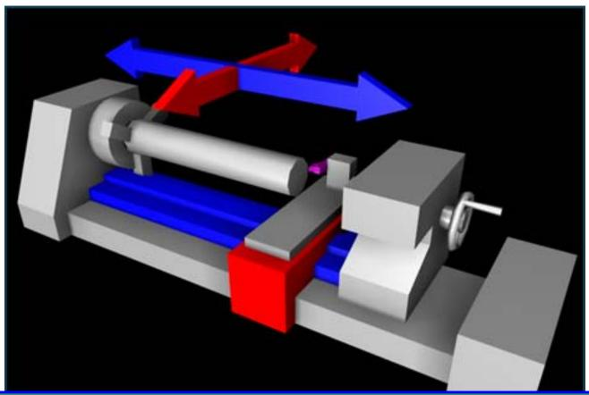
On most CNC lathes the Z A is is parallel to the spindle and longer than the X Axis.
