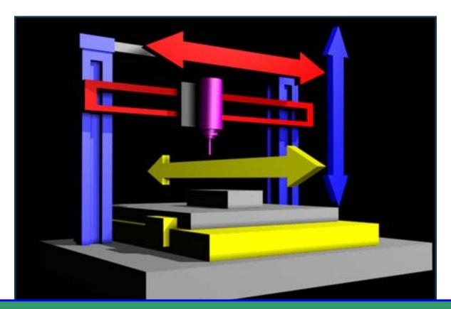
On this gantry mill the spindle travels along the **X** Axis. The travel direction of the table designates the **Y** Axis. The **Z** Axis is designated by the stationary vertical column.
