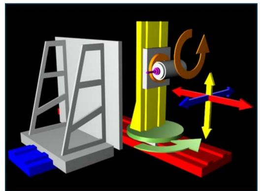
On this five-axis horizontal contour milling machine, note the orientation of the  $\mathbf{X}$  and  $\mathbf{Y}$  axes in relation to the  $\mathbf{Z}$  Axis. The rotary axes for both the  $\mathbf{X}$  and  $\mathbf{Y}$  axes are designated by the  $\mathbf{A}$  and  $\mathbf{B}$  rotary tables.
