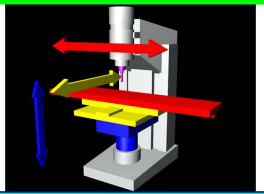
On a common vertical knee CNC mill the spindle is stationary while the rest of the components move according to their axis designations ( $\mathbf{X}, \mathbf{Y}$ , and  $\mathbf{Z}$ ).
