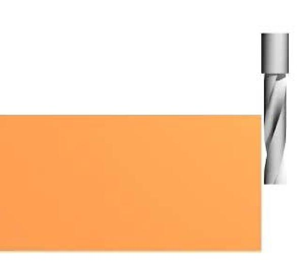
Linear Interpolation, or straight-line feed moves, on the flat XY plane (no Z values are specified).
