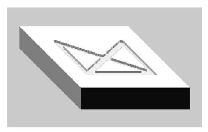
Workpiece Size: X5, Y4, Z1 Tool: Tool #2, 1/4" End Mill Tool Start Position: X0, Y0, Z1 (Relative to workpiece) % :1002 N5 G90 G20 N10 M06 T2 N15 M03 S1200 N20 G00 X1 Y1 N25 Z0.125 N30 G01 Z-0.125 F5 N35 X4 F10 N40 Y3 N45 X1 Y1 N50 Y3 N55 X4 Y1 N60 G00 Z1 N65 X0 Y0 N70 M05 N75 M30
