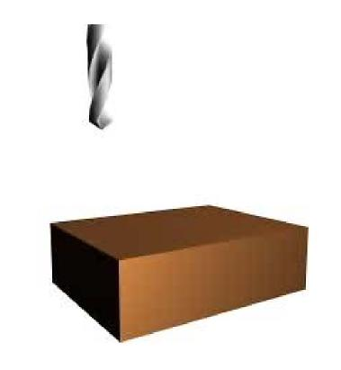
In the G83 cycle, Q is the incremental depth of cut.
