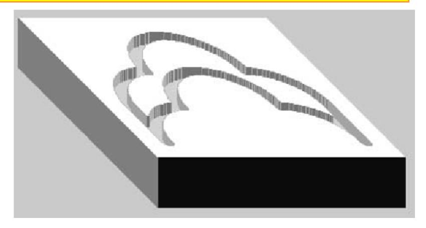
Workpiece Size: X5, Y4, Z1 Tool: Tool #2, 0.25" Slot Mill Tool Start Position: X0, Y0, Z1 (Relative to workpiece) % :1003N5 G90 G20 N10 M06 T2 N15 M03 S1200 N20 G00 X0.5 Y0.5 N25 Z0.25 N30 G01 Z-0.25 F5 N35 G02 X1.5 Y1.5 I1 J0 F10 N40 X2.5 Y2.5 R1 N45 X3.5 Y1.5 I0 J-1 N50 X4.5 Y0.5 R1 N55 G01 Y1.5 N60 G03 X3.5 Y2.5 R1 N65 X2.5 Y3.5 I-1 J0 N70 X1.5 Y2.5 R1 N75 X0.5 Y1.5 I0 J-1 N80 G01 Y0.5 N85 G00 Z1 N90 X0 Y0 N95 M05 N100 M30
