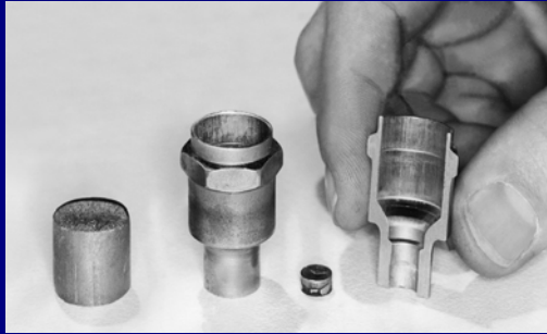
Production steps for a cold extruded spark plug
